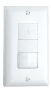
The IR VS 1 is a line voltage, single relay, Passive Infrared (PIR) wall switch vacancy (manual ON) sensor intended to control lighting in commercial spaces. PIR is used where the sensor will have a clear view of the occupants in the desired coverage area. The convenient "Switch Link" feature enables up to four sensors to link together for peer to peer grouping achieving expanded detection zones and multiway switching.
